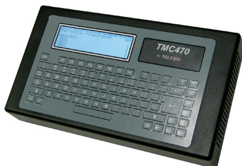
Compact Self-Contained TMC470 Controller — no PC required.
